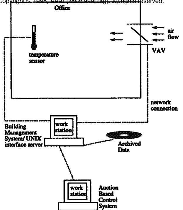
Fig. 1. Schematic diagram of the instrumentation in an office and the connections to the computerized auction.
